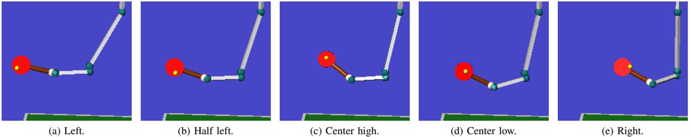
Figure 9: This figure shows samples of the learned forehands. Note that this figure only illustrates the learned meta-parameter function in this context but cannot show timing and velocity and it requires a careful observer to note the important configuration differences resulting from the meta-parameters.
