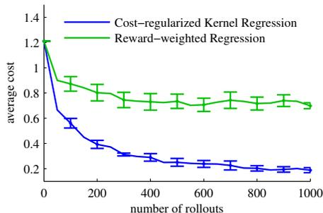
Figure 6: This figure shows the cost function of the dart-throwing task for a whole game *Around the Clock* in each rollout. The costs are averaged over 10 runs with the error-bars indicating standard deviation.
