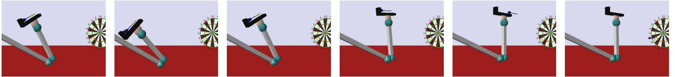
(a) The robot is in the rest posture and the dart is placed on the launcher. (b) The arm moves back. (c) The arm moves forward on an arc. (d) The arm stops. (e) The dart is carried on by its momentum. (f) The dart hits the board.
