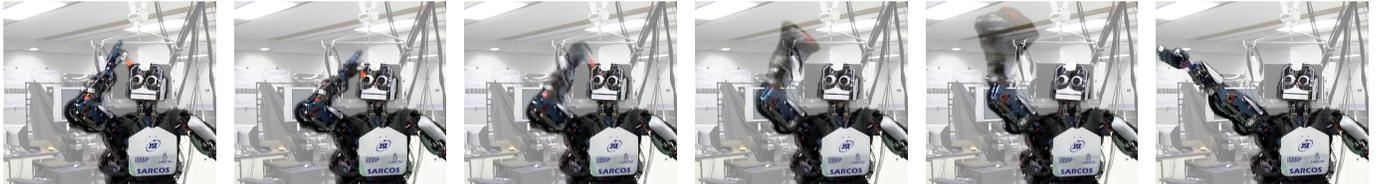
(a) The robot is in the rest posture and the dart is placed in its hand. (b) The arm moves back. (c) The arm moves forward on an arc. (d) The arm continues moving. (e) The dart is released and the arm follows through. (f) The arm stops and the dart hits the board.
