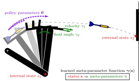
Figure 1: This figure illustrates a 2D dart throwing task. The situation, described by the state  $s$  corresponds to the relative height. The meta-parameters  $\gamma$  are the velocity and the angle at which the dart leaves the launcher. The policy parameters represent the backward motion and the movement on the arc. The meta-parameter function  $\gamma(s)$ , which maps the state to the meta-parameters, is learned.
